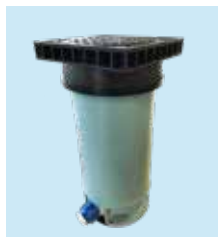
SERIES 8054/6211 Water Meter Boundary Box Grade C version BS 5834-1:2017 PN16 d20-32, ¾" BSP, ½" HG Square PP frame
