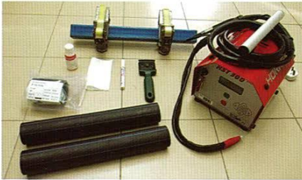
[ 1 ] Prepare the electrofusion welding unit and other ancillary equipment.
