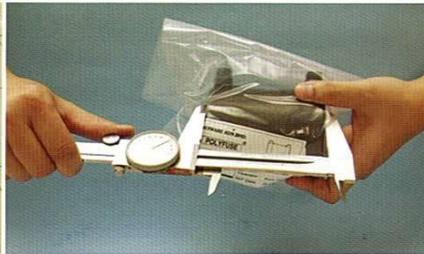
[ 2 ] Measure the total length of the fitting.
